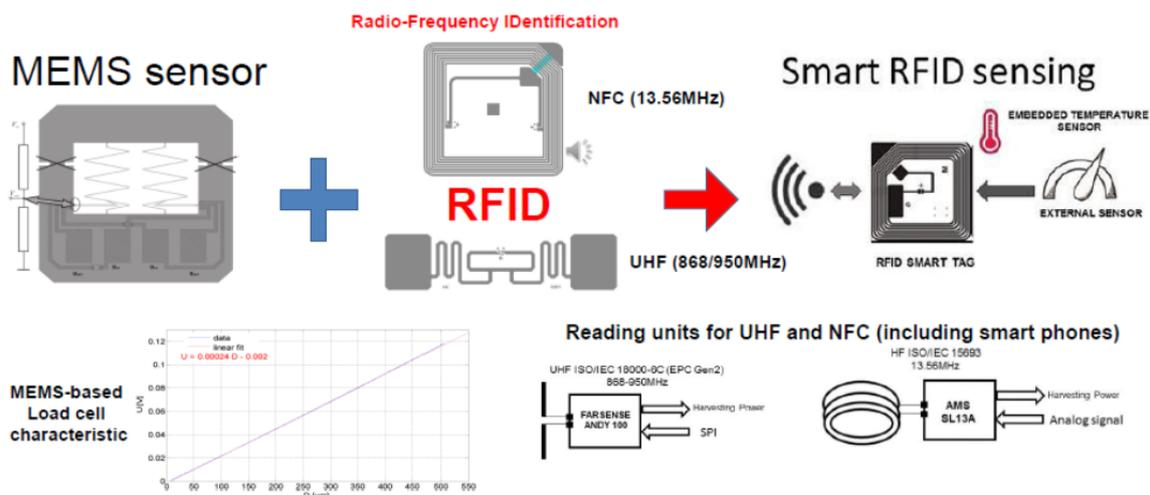
The University - EPU has developed a technology for off-chip contactless sensor communication via RFID standard channels. This technology provides the opportunity to upgrade the existing MEMS sensors with a contactless (wireless) remote data exchange capability without a change of the chip (sensor) design. It is done by in-sensor package incorporating of the RFID infrastructure, which is capable to process and transmit both digital or analog sensor signals.
