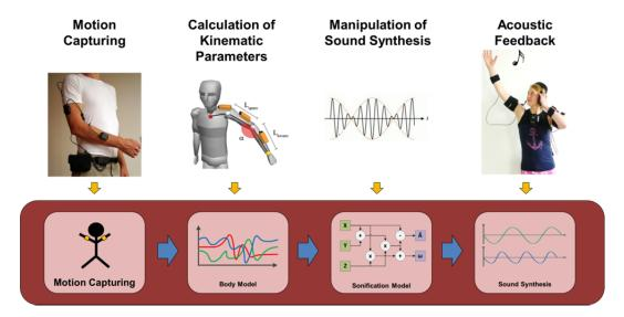
For a reliable sonification of movements a highly accurate motion capturing system has to be used. Camera-based systems which are well known as highly reliable require a stationary setup and a permanent line of sight between the tracked objects and multiple cameras. In contrast, mobile and wearable inertial sensors can be easily attached to the human body [8]. This is mandatory for human motion capturing in sport training sessions or medical applications.
