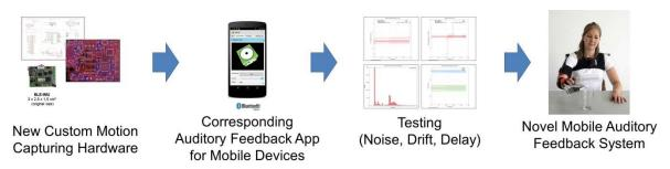
The system is comprised of multiple motion capturing units and a smart phone. The motion capturing units transmit their sensor data to the smartphone via Bluetooth Low Energy. Sensor fusion, combination of the calculated orientation(s) with the body model and sonification downstream are performed on the smart phone resulting in a compact and affordable system.
