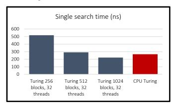
Results do not show a great performance improvement, but this implementation let us identifying the optimal tradeoff e.g., between CUDA threads/blocks. Subsequently, we applied **CompactArr**, an original memory allocator developed by us in the domain of a previous research project named LightKer, and further optimizing the code, achieving a final speedup of 8x compared to CPU-based implementation, and a 2-3x reduction in the memory footprint of the Sensigrafo.
