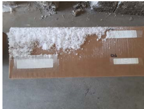
Fig. 3: One of the tagged boxes after the three-month exposure. One of the tags selected during the TP works properly even if covered by ice.
