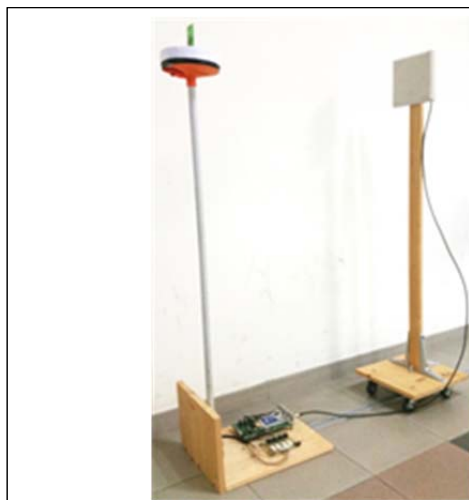
Fig. 1: Measurement system for RFID tags performance evaluation
