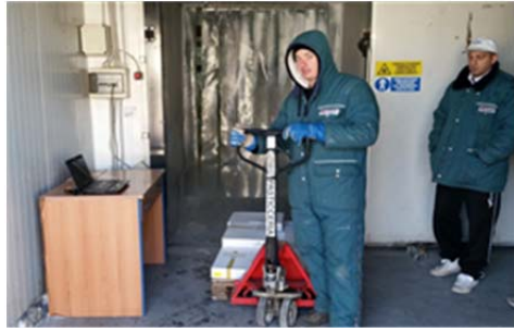
Fig. 3: Cold room entry. The most critical step in the Martinucci's supply chain is the storage in the cold rooms, because of the very low temperature (-27 °C) that can impact on the performance of both RFID readers and tags.
