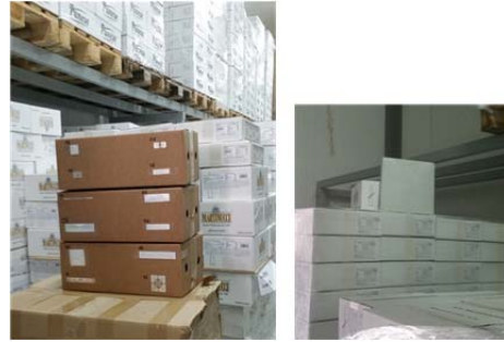
Fig. 4: RFID tags applied on cake boxes and stored in the cold room along with a reader antenna. Some tags did not change their performance at all after a three-month exposure.
