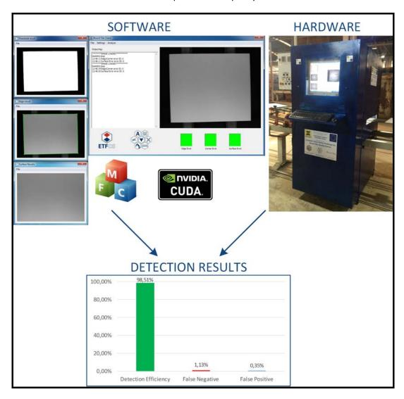
In this TTP, we are designing computer vision station prototype based on mechanical construction or housing and computer vision system with camera, lighting, and industrial computer. Prototype system is developed for production line in ceramic tiles factory for detection of edge defects, corner
